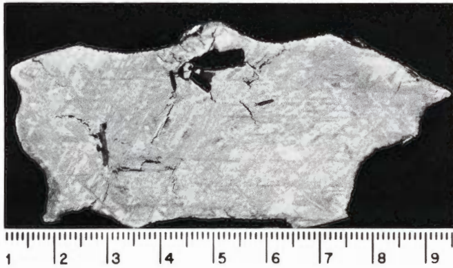
Figure 346. Bishop Canyon (Tempe no. 360.1). Endpiece of 198 g showing large silica inclusions, which are highly unusual in group IVA. Etched. Scale bar in cm. (Courtesy C.B. Moore.)
