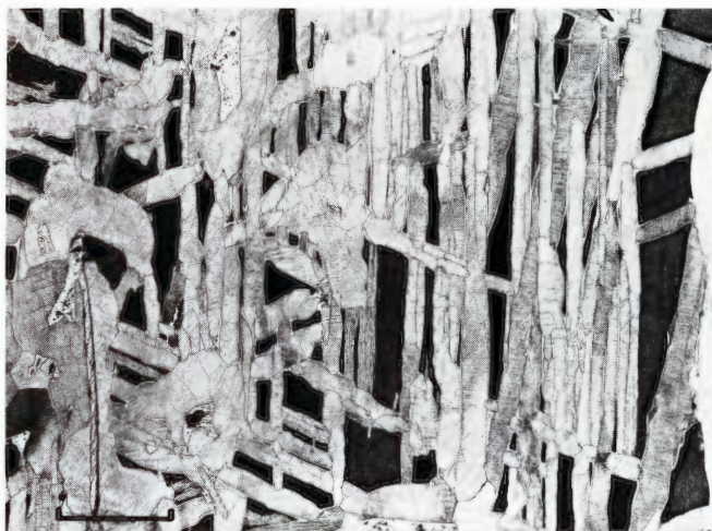
Figure 328. Bella Roca (Copenhagen no. 1891, 53). General view at low magnification. The shock-hatched kamacite displays various nuances. Large skeleton crystals of schreibersite are common. Deep-etched. Scale bar 300 \mu .
