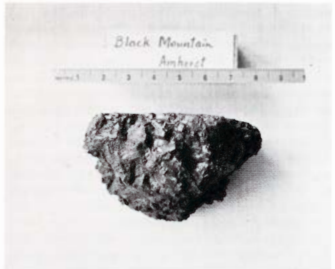
Figure 355. Black Mountain (Amherst). The weathered 351 g endpiece is the largest fragment preserved of this controversial meteorite which may be a transported sample of Duel Hill (1873). Scale bar in cm.
