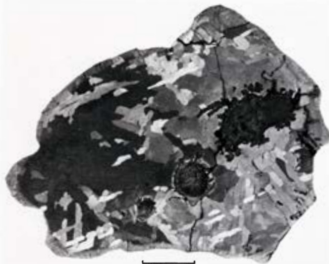
Figure 361. Bogou (U.S.N.M. no. 2245). A full, deep-etched slice. The heat-affected \alpha_2 rim zone is distinctly seen: wide under the knobs, but narrow at the bottom of regmaglypts. Large troilite-graphite-silicate aggregates with rims of schreibersite and cohenite. A few cohenite crystals are in the kamacite lamellae to the extreme right. Scale bar 20 mm. S.I. neg. M-1375A.
