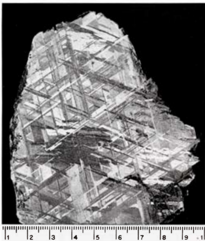
Figure 375. Bristol (Tempe no. 216.14). A general view of the fine octahedrite which is closely related to Gibeon. Etched. Scale bar in cm. (Courtesy C.B. Moore.)
