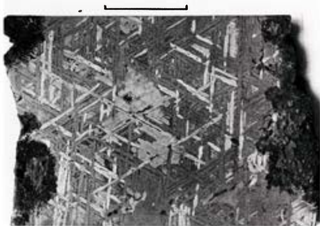
Figure 372. Bridgewater (Helsinki no. A 2318). Cut almost parallel to (111) \gamma . Strong oriented sheen in the Widmanstätten structure. Millimeter-sized schreibersite crystals with rims of swathing kamacite. Terrestrial corrosion (black). Deep etched. Scale bar 20 mm.
