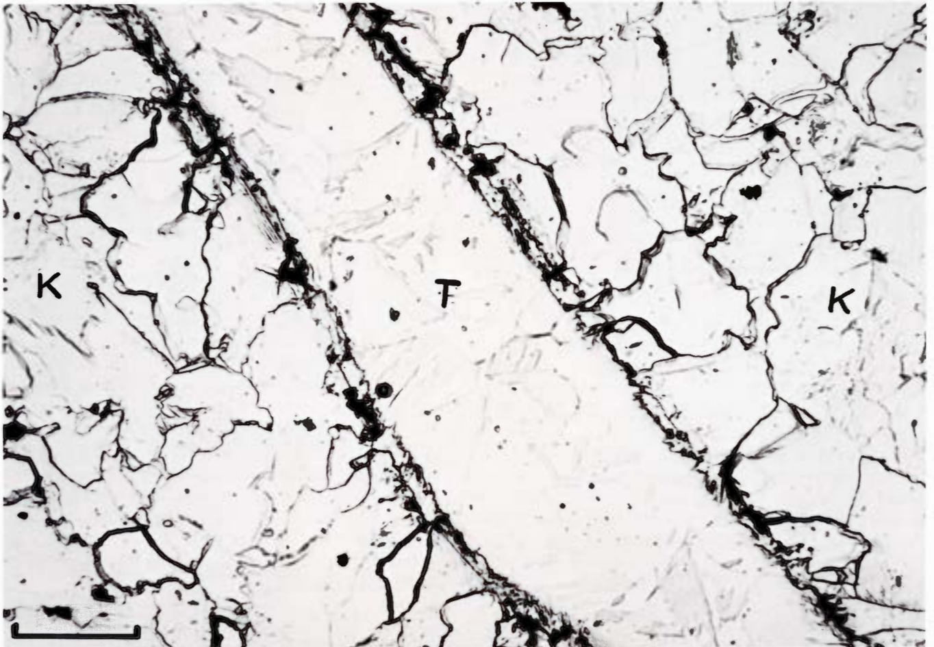
Figure 387. Burlington (U.S.N.M. no. 978). Detail of a kamacite lamella (T) between two kamacite lamellae (K). All transformed to \alpha_2 , however, of different morphology because of high nickel content in the taenite and low in the kamacite. Etched. Scale bar 40 \mu . See also Figure 27A.
