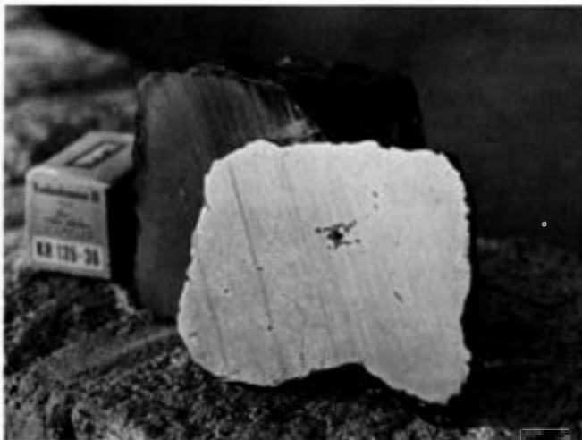
Figure 422. Calico Rock. Main mass in the background and a full slice in front. The box-like shape is clearly seen. The exterior faces are parallel to (100)_{\alpha} , the cubic cleavage planes. The side of the film box is 4 cm. S.I. neg. M-1296A.
