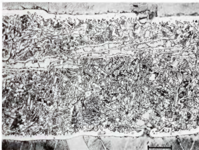
Figure 419. Cachiyual (Chicago no. 958). General appearance of an annealed plessite field. The cloudy taenite rims have disappeared. Etched. Scale bar 50 \mu .
