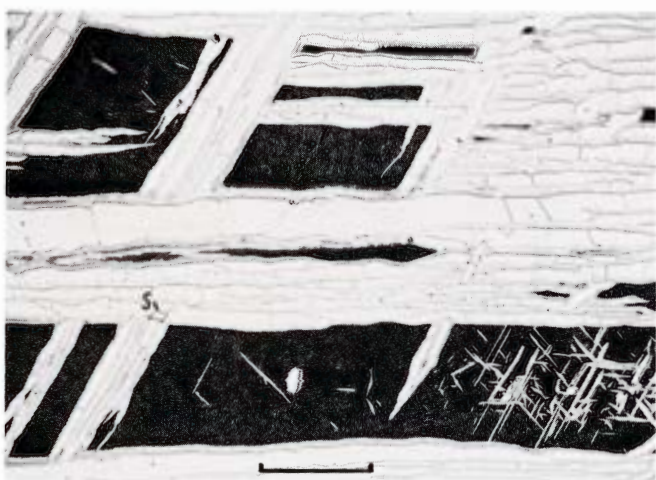
Figure 404. Butler (Harvard no. 354). An area rich in relatively coarse kamacite spindles. Schreibersite (S). Compare Figure 405 with the same magnification. Etched. Scale bar 500 \mu . (Perry 1950: volume 1.)
