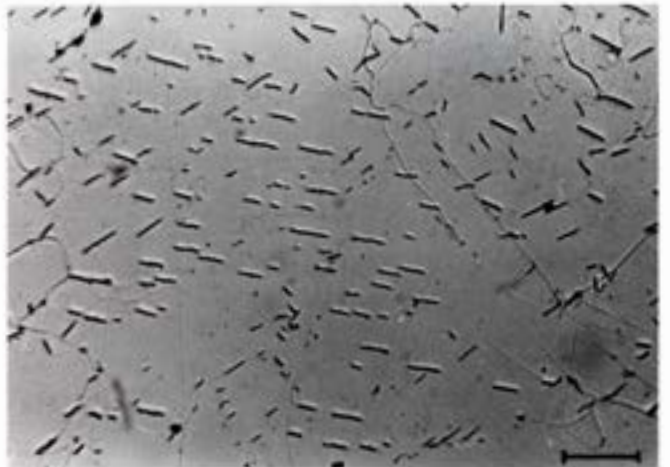
Figure 415. Cacaria (Tempe no. 19a). Detail of Figure 414. The oriented platelets in the ferrite are perhaps nitrides. Etched. Scale bar 20 \mu .
