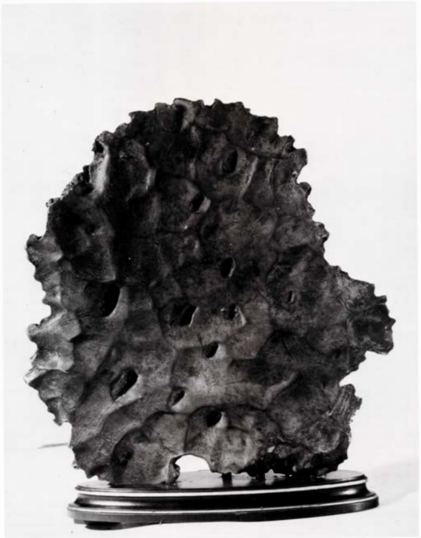
Figure 409. Cabin Creek. The rear side of the main mass in Vienna. Shallow, large regmaglypts and depressions from ablated troilite nodules. The height of the specimen is 44 cm. (Courtesy Dr. Gero Kurat, Vienna.)
