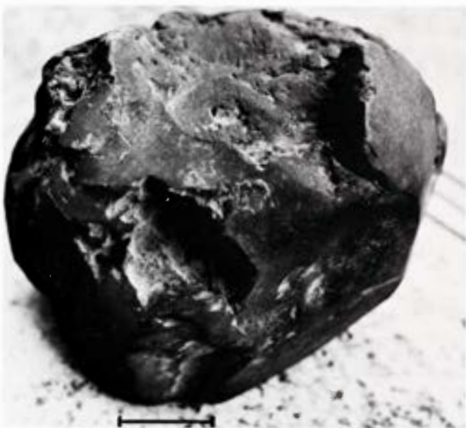
Figure 410. Cacaria. Main mass in Museum de Chopo, Mexico City. Its exterior shape has been significantly altered by forging in which some kind of a drop hammer was used. Scale bar 5 cm.
