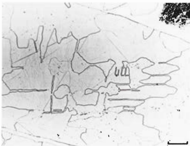
Figure 427. Cambria (Tempe no. 359.1). Partially recrystallized area. Original Neumann bands are still visible. Etched. Scale bar 50 \mu .
