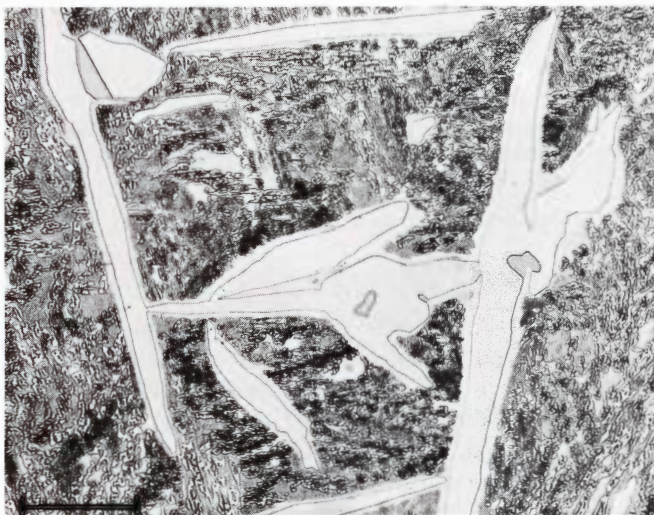
Figure 406. Butler (Copenhagen no. 1876, 2247). The black matrix is at high resolution seen to be composed of minute \alpha + \gamma particles. Widmanstätten \alpha -spindles are associated with three schreibersite particles. Etched. Scale bar 50 \mu .
