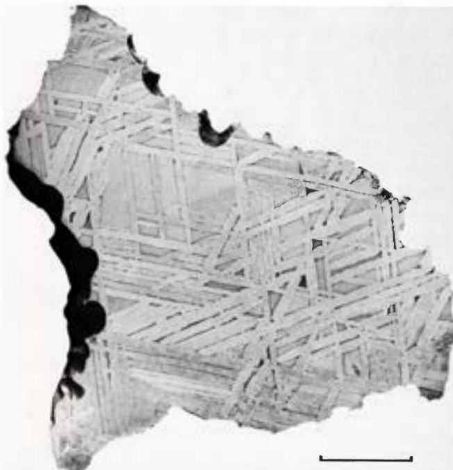
Figure 418. Cachiyual (Chicago no. 958). Deep-etched section showing the regular Widmanstätten structure. Since the kamacite is recrystallized there is no oriented sheen. Scale bar 20 mm. S.I. neg. M-650B.
