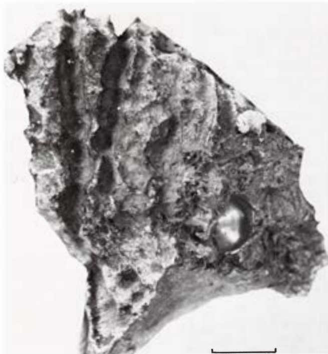
Figure 417. Cachiuyual (Chicago no. 958). The main mass with its characteristic pitting corrosion from exposure to the Atacama climate. Drill-hole for analysis below right. Scale bar 20 mm. S.I. neg. M-650A.
