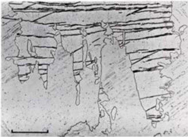
Figure 413. Cacaria (Tempe no. 19a). In near-surface areas mechanical deformation twins, resembling Neumann bands, are quite common. They must have been caused by heavy machine blows. Etched. Scale bar 100 \mu .
