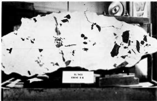
Figure 433. Campo del Cielo. The El Taco mass being cut in Mainz. Numerous large angular silicate-troilite-graphite aggregates. Length of slice 110 cm. (Courtesy Professor Hintenberger.) See also Figure 78.
