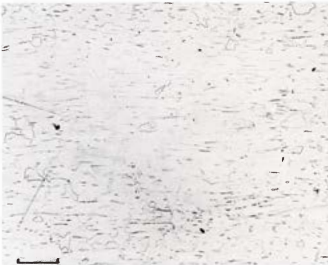
Figure 431. Campo del Cielo, labeled Otumpa (Copenhagen no. 2). The sample has, like much of the old Campo del Cielo material, been artificially reheated and partially forged. The indistinct horizontal lines suggest inhomogeneities after partial resorption of rhabdites and taenite. \alpha_2 matrix. Etched. Scale bar 300 \mu .
