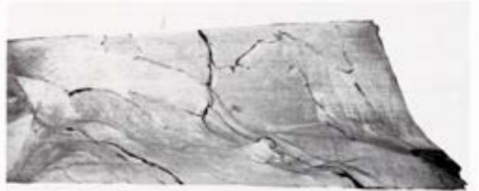
Figure 436. Campo del Cielo (U.S.N.M. no. 2253). Section through a mass that was heavily coldworked when the meteorite split in the atmosphere. Wavy sliplines and deformation bands cross the entire specimen. Etched. Scale bar 3 mm. S.I. neg. 1358G.
