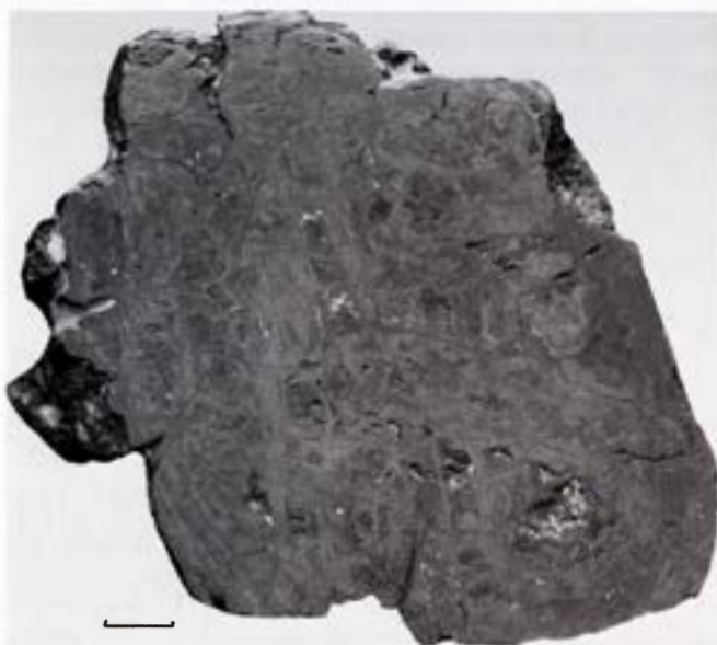
Figure 477. Canyon Diablo. Section through an angular shapeless oxide ball. Small unweathered meteorite particles, mainly of taenite and schreibersite, may be seen as white specks in the limonite. Polished. Scale bar 10 mm. S.I. neg. M-951.
