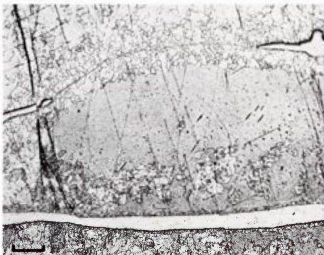
Figure 481. Canyon Diablo. The Helt Township sample (U.S.N.M. no. 1323). The microstructure corresponds closely to that of shock-annealed samples of stage IV. Compare Figures 461-465. Etched. Scale bar 100 \mu . (Perry 1950: volume 2.)
