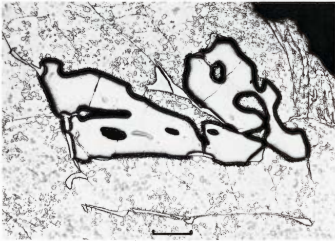
Figure 470. Canyon Diablo. Stage VI, as Figure 469. The cohenite crystals, Figure 469, show distinct black rims, and the kamacite displays unequilibrium \alpha_2 . Scale bar 500 \mu .
