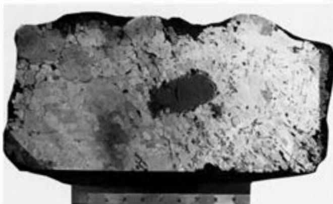
Figure 668. Cosby's Creek (Harvard no. 143). In the center, a troilite nodule. To the right cohenite-rich kamacite. Deep-etched. Scale bar in centimeters.
