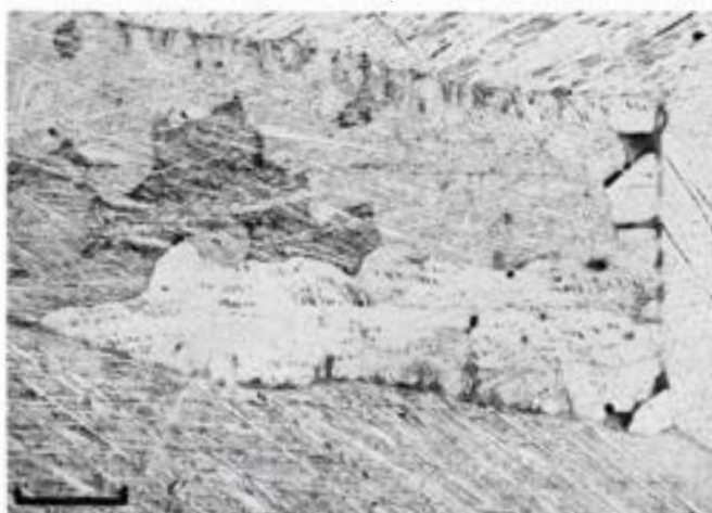
Figure 670. Costilla Peak (Tempe no. 190.1). Open-meshed plessite field with shock-hatched kamacite of various shades. Etched. Scale bar 200 \mu .
