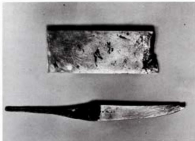
Figure 750A. Elbogen (Humboldt University, Berlin). Above a piece which, after polishing, has been slightly heated so that the Widmanstätten pattern is developed in purple, blue and yellow colors (German Anlaufätzung, English heat-tinting). Below, a knife, 83 mm long, forged from Elbogen material. Both specimens originally in the possession of Chladni. (Courtesy Professor G. Hoppe.)
