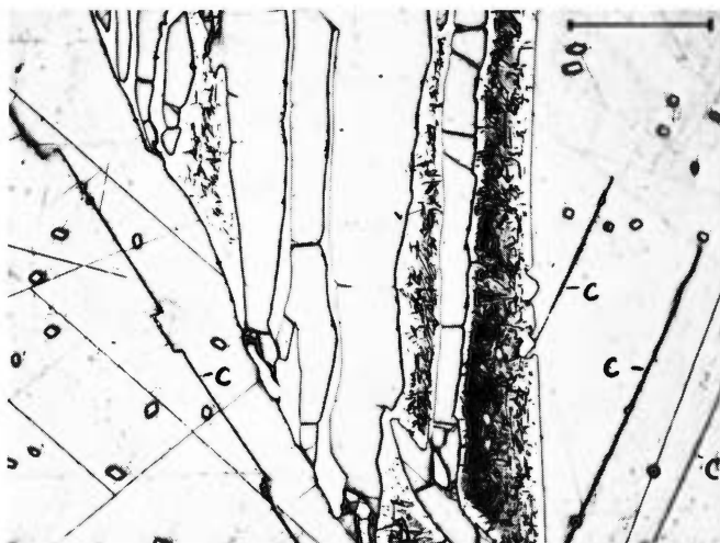
Figure 759. Emsland (Copenhagen no. 1973, 2081). The cleavage cracks (C) follow (100)_\alpha planes in the kamacite lamellae. Thin black lines indicate Neumann bands. Acicular pleistite fields and conspicuous rhabdites. Etched. Scale bar 200 \mu .
