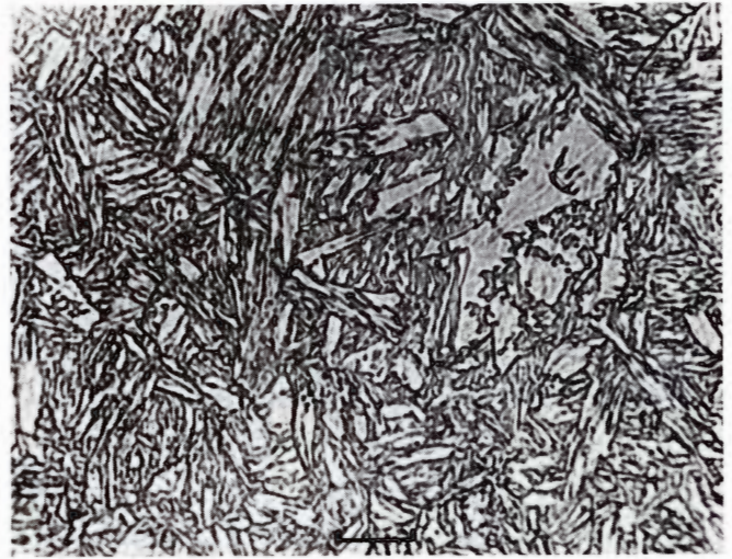
Figure 766. Föllinge (Stockholm no. 335,317b). The plessitic fields of Figure 763 reveal, upon heating etching, martensitic structures. The orientation is random, in sharp contrast to the (111) \gamma martensite platelets of unheated meteorites. See, e.g., Figures 690 and 816. Scale bar 10 \mu .
