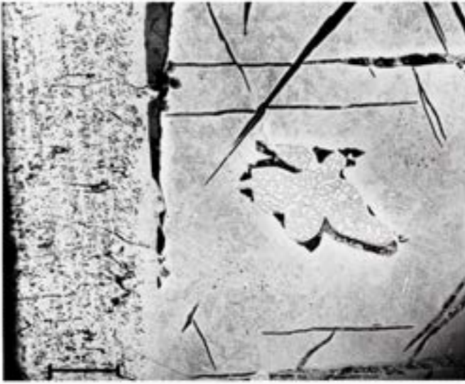
Figure 764. Föllinge (Stockholm no. 335,317b). To the left a layered fusion crust. To the right the heat-affected \alpha_2 zone (A) with a fused schreibersite crystal. Terrestrial corrosion has selectively converted some kamacite lamellae to limonite (black). Etched. Scale bar 300 \mu .
