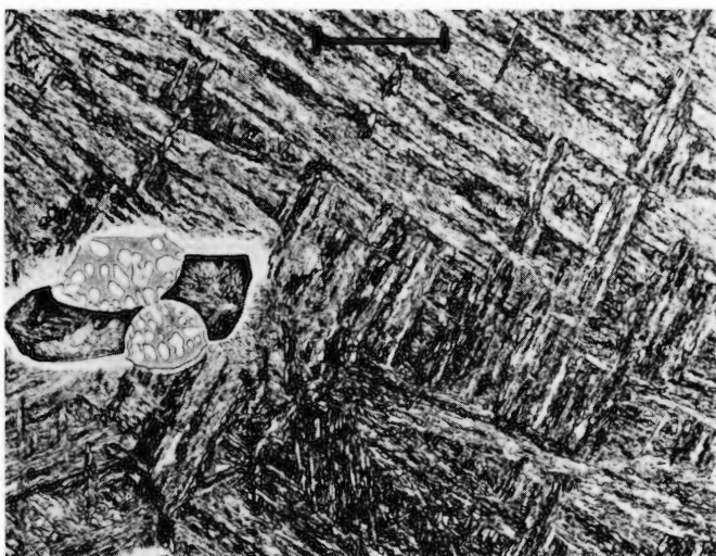
Figure 774. Freda (U.S.N.M. no. 1342). Heat-affected A-zone with fused schreibersite crystals. Etched. Scale bar 40 \mu . (From Henderson & Perry 1942.)
