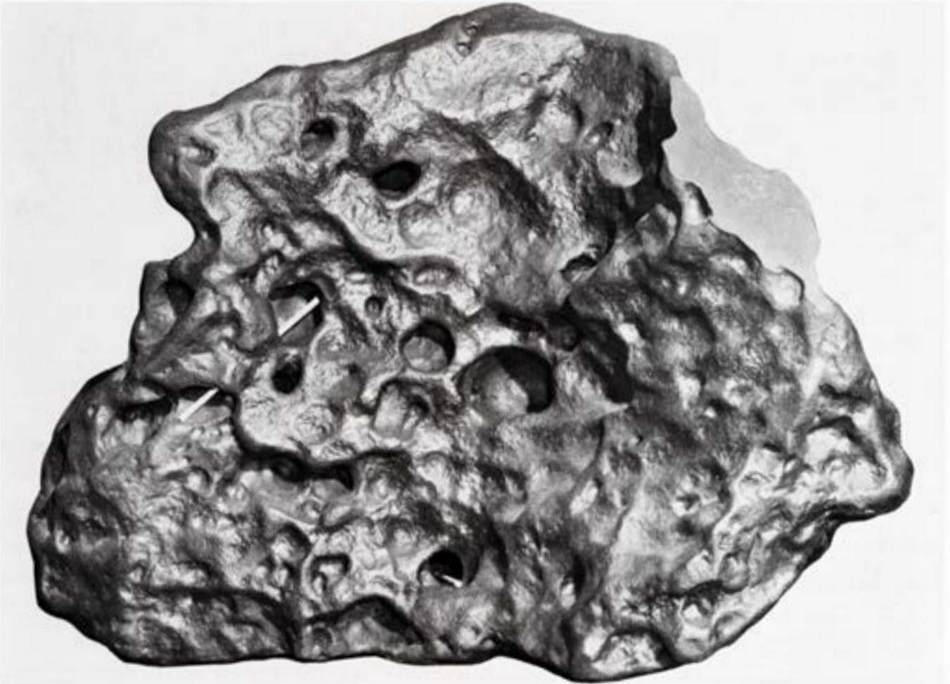
Figure 802. Goose Lake (U.S.N.M. no. 1332). The 1,163 kg main mass with its characteristic and enigmatic cavities. The white ruler measures 20 cm and is inserted in two connecting cavities. Below, another ruler is inserted into a hole which connects with the large cavity on the opposite side. Above right, a 30 x 10 cm cut indicates from where the only material for examination has been taken. S.I. neg. 41402.
