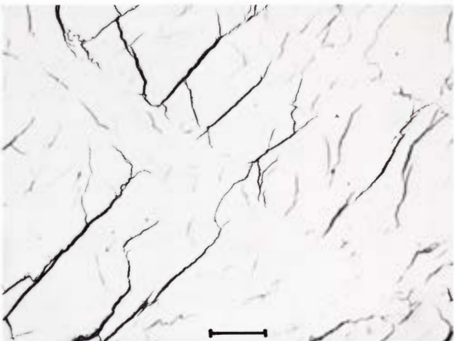
Figure 818. Grant (U.S.N.M. no. 836). A Brezina lamella of schreibersite. Most of the schreibersite lamellae are similarly cracked, probably a result of the same shock event that hardened the kamacite and taenite. Polished. Scale bar 50 \mu .
