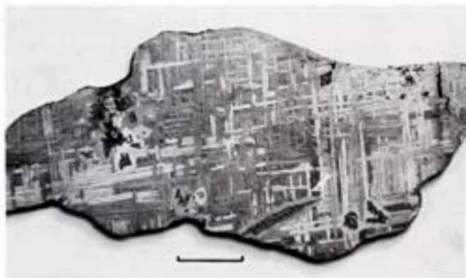
Figure 804. Goose Lake (U.S.N.M. no. 1332). The section is almost parallel to (100) \gamma and, therefore, shows only two sets of Widmanstätten lamellae, almost perpendicular to each other. Troilite-graphite-silicate nodule to the left, and many large skeleton crystals of schreibersite. These are enveloped by narrow cohenite rims (black) and swathing kamacite. The thin, dark veins are terrestrial corrosion products. Deep-etched. Scale bar 30 mm. S.I. neg. 37144.
