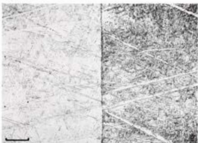
Figure 817. Grant (U.S.N.M. no. 836). Shock-hatched kamacite. Slightly different development in two adjacent kamacite lamellae because they are oriented differently. Etched. Scale bar 50 \mu .
