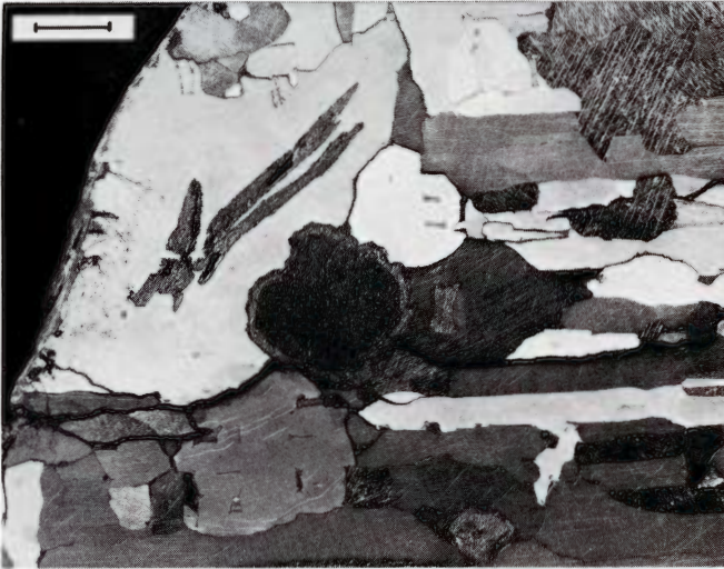
Figure 876. Hope (U.S.N.M. no. 3476). Grain growth of kamacite has engulfed former Widmanstätten taenite fields. Schreibersite skeleton crystals with cohenite rims and wide zones of swathing kamacite. Deep-etched. Scale bar 5 mm. S.I. neg. 1519B.
