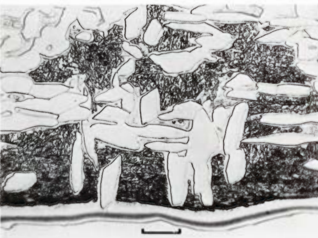
Figure 883. Hopewell Mounds (Chicago no. 481). Cloudy taenite rim with duplex unresolvable transition zones to interior net plessite. Etched. Scale bar 20 \mu .
