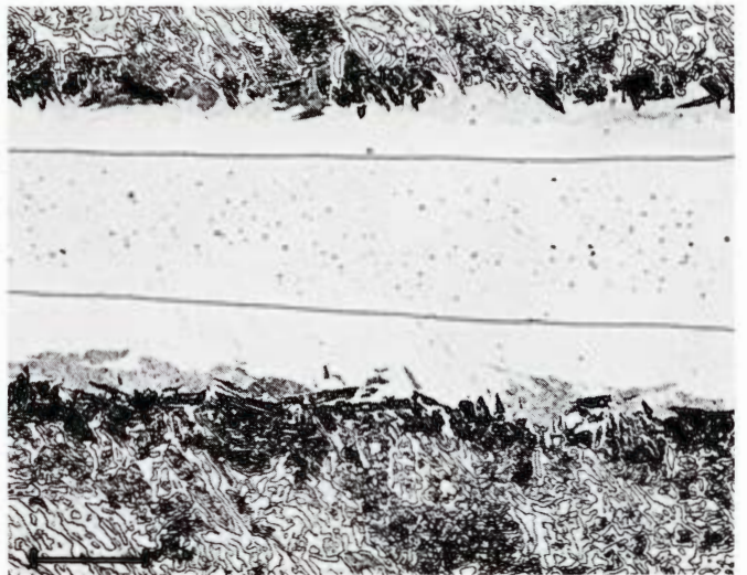
Figure 866. Hoba (New York no. 2681). A kamacite spindle enveloped in taenite, unresolvable transition zones and easily resolvable duplex \alpha + \gamma mixtures. Etched. Scale bar 20 \mu . (Perry 1950: volume 2.)
