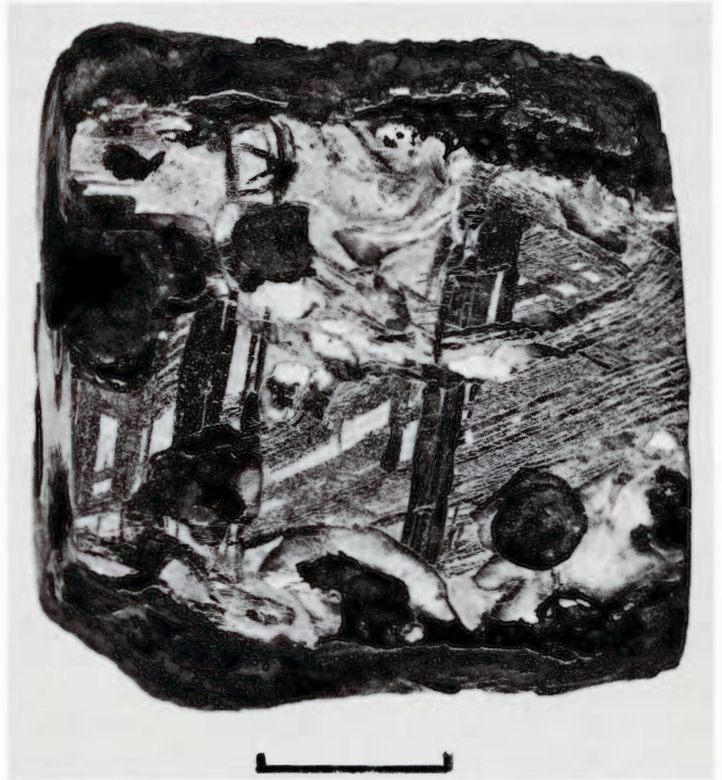
Figure 877. Hopewell Mounds (Chicago no. 480; 103 g). Cold-worked sample with olivine inclusions. Deep-etched. Scale bar 2 cm. S.I. neg. 37839.
