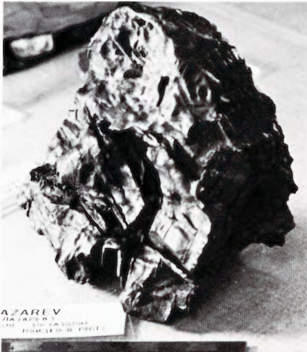
Figure 1047. Lazarev (Moscow). The 2 kg mass in Moscow. The weathered meteorite displays a distinct Widmanstätten grid on part of the surface. Octahedral fissures are present. Ruler divided in cm.
