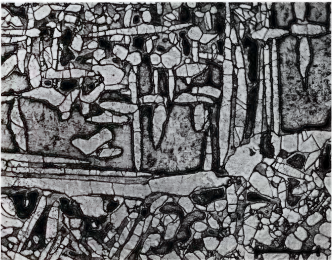
Figure 1064. Linville (U.S.N.M. no. 551). The horizontal kamacite band is located along a former \gamma\gamma grain boundary. The two original taenite crystals are randomly oriented as may be deduced from the Widmanstätten patterns. The kamacite is transformed to unequilibrated \alpha_2 by artificial reheating. Etched. Scale bar 200 \mu . (Perry 1950: volume 3.)
