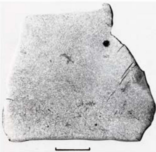
Figure 1079. Locust Grove (Vienna no. G8418). An 8 mm thick slice, somewhat flattened by forging. The structure is entirely altered from that of a normal hexahedrite, due to artificial reheating above 1000° C. Deep-etched. Scale bar 20 mm.
