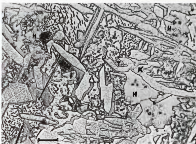
Figure 1198. Mungindi (U.S.N.M. no. 2944). A photograph with maximum contrast between kamacite (K), taenite (T) and haxonite (H). Etched. Scale bar 10 \mu .
