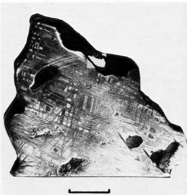
Figure 1193. Mungindi (Prague no. 120). A fine octahedrite of group IIIC. Troilite nodules with schreibersite rims and well-preserved exterior surface. Deep-etched. Scale bar 20 mm.
