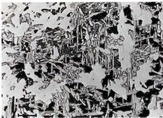
Figure 1195. Mungindi (U.S.N.M. no. 2944). Detail of an acicular plessite field with haxonite precipitates (white). Scattered phosphides are also present. Compare Figure 1196. Etched. Scale bar 50 \mu . See also Figures 144A and 144B.
