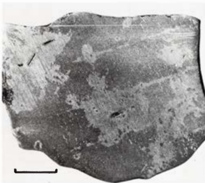
Figure 1202. Murphy (Vienna no. H976). A one centimeter thick full slice. Deep-etching develops the characteristic pattern of light (rhabdite-poor) and dark (rhabdite-rich) patches. Troilite-schreibersite inclusions are located centrally in the light areas. Scale bar 20 mm.
