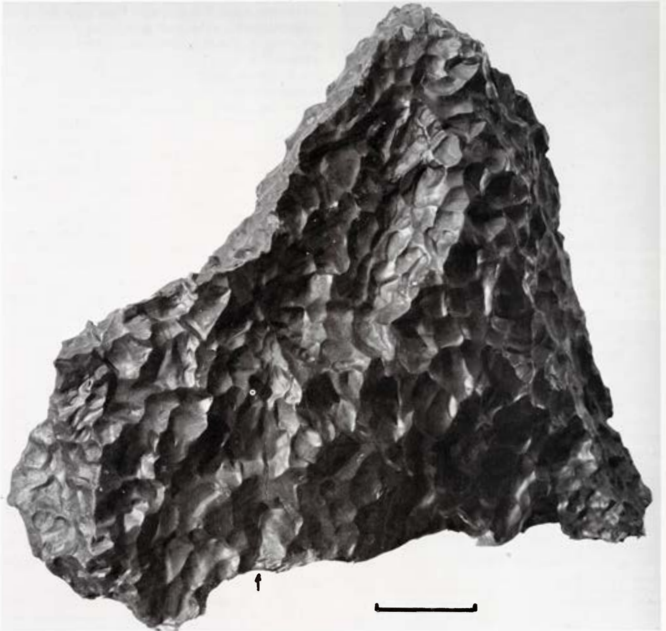
Figure 1201. Murnpeowie. The eminent main mass of 1,140 kg in Adelaide. Regmaglypts, and a fine crack just above the arrow. Scale bar approximately 20 cm.
