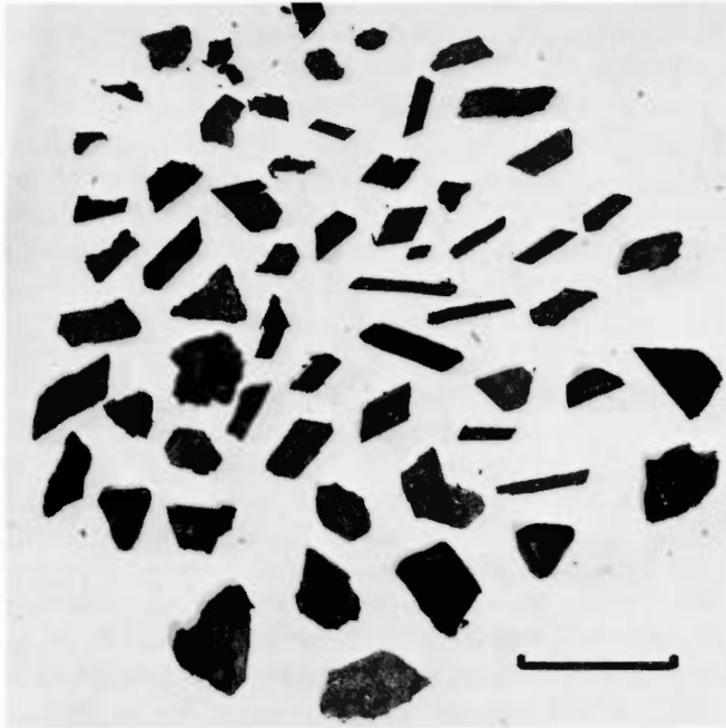
Figure 1218. Nashville (U.S.N.M. no. 894). The disintegrated fragments suggest that the original meteorite was an octahedrite. Scale bar 40 mm.
