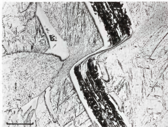
Figure 1217. Narraburra (Copenhagen no. 1905, 1732). A cosmic collision-event shock-hardened the kamacite and taenite and locally caused heavy shear-displacement. Here a faulted plessite field. Etched. Scale bar 100 \mu .
