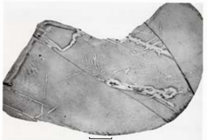
Figure 1206. Muzzaffarpur. Same as Figure 1205 with the light source in a different position. The kamacite spindles are clearly distinguished. Scale bar 5 mm. S.I. neg 1061.
