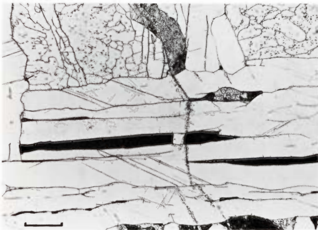
Figure 1307. Obernkirchen (U.S.N.M. no. 1611). A fine octahedrite of group IVA. Within a vertical shear zone the kamacite is recrystallized. Etched. Scale bar 500 \mu .
