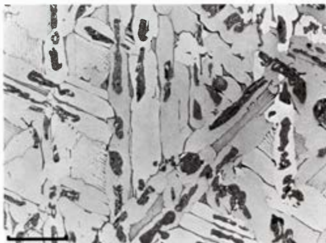
Figure 1314. Odessa. Detail of Figure 1312. Elongated cohenite crystals with "windows" of kamacite, taenite and schreibersite. Various plesite fields. Deep-etched. Scale bar 5 mm. S.I. neg. 1343D.
