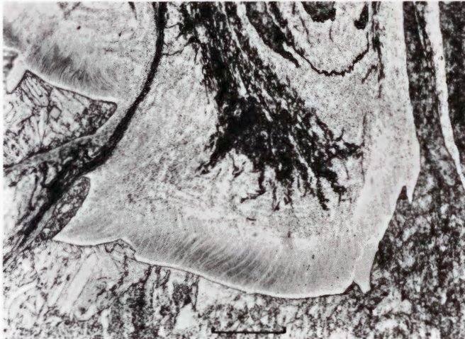
Figure 1407B. Puquios (U.S.N.M. No. 153). Detail of a shear zone with very heavy displacements. The central plessite field shows altered taenite rims with distinct striping caused by violent deformation. Etched. Oil immersion. Scale bar 20 \mu .
