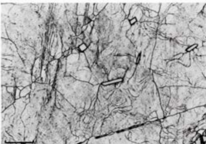
Figure 1399. Providence (U.S.N.M. no. 2568). Angular prismatic rhabdites in kamacite rich in subboundaries. Etched. Scale bar 100 \mu .
