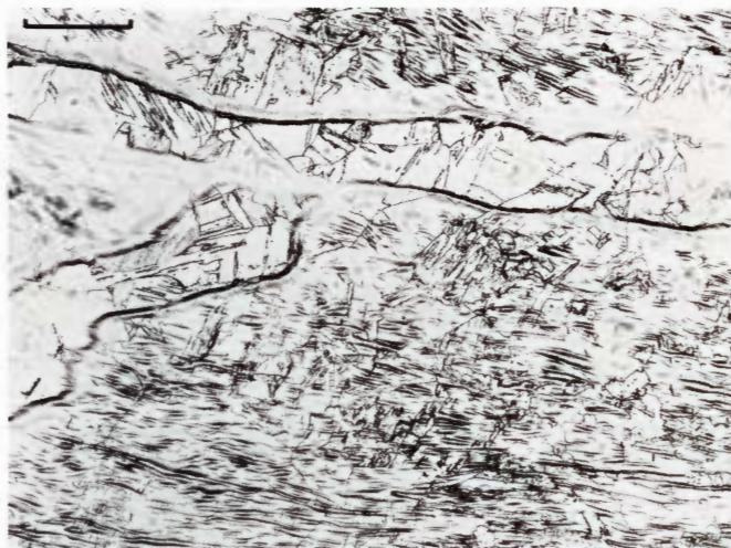
Figure 1392. Prambanan (Chicago no. 1,160). Artificially altered structure. The parallel horizontal ghost-lines indicate forging. All kamacite has been through the \alpha \rightarrow \gamma \rightarrow \alpha_2 transformation. The plesite fields show diffuse interfaces with kamacite. Etched. Scale bar 200 \mu . See also Figure 132.
