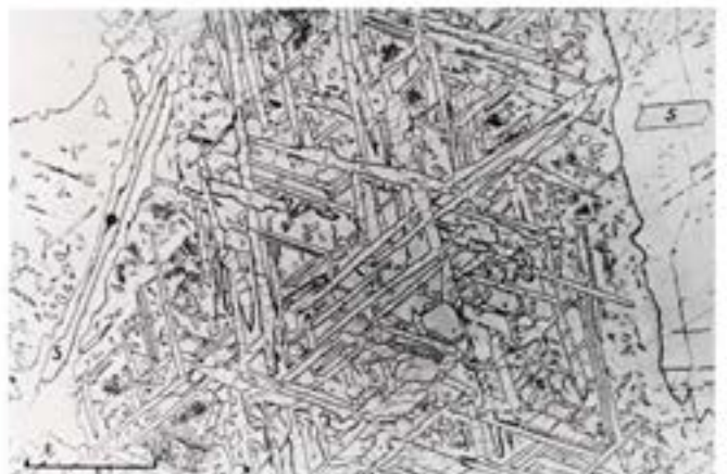
Figure 1486. Saint Francois County (Tempe no. 173a). Annealed acicular plessite field with scattered phosphide inclusions (S). The kamacite is subdivided in cells. Etched. Scale bar 100 \mu .
