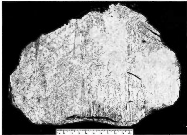
Figure 1469. Ruff's Mountain (Tempe no. 99b). A recrystallized medium octahedrite transitional between group IIIA and IIIB. Deep-etched. Scale in centimeters. (Courtesy C.B. Moore.)
