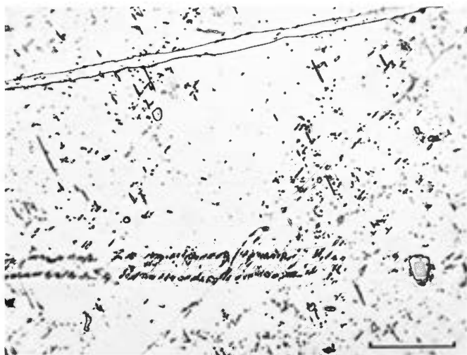
Figure 1574. Seeläsgen (Copenhagen no. 32). Three annealed Neumann bands, one of them with a rhabdite (right) showing a reaction halo of taenite. Fine needles in the matrix, probably of isothermal taenite caused by the annealing. Etched. Scale bar 30 \mu .
