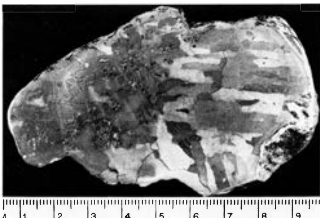
Figure 1575. Seligman (Tempe no. 583.3). A coarse octahedrite of group I. Cohenite crystals in the left part. Deep-etched. Scale in centimeters. (Courtesy C.B. Moore.)
