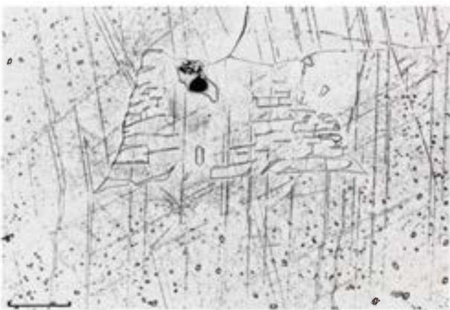
Figure 1567. Seeläsgen. Detail of Figure 1566 showing a degenerate comb plessite field with a schreibersite crystal. Annealed Neumann bands and rhabdites are common. Etched. Scale bar 300 \mu .
