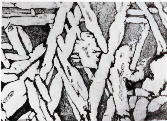
Figure 1580. Seneca Falls (Chicago no. 60). A recrystallized medium octahedrite of group IIIA. Several schreibersite crystals in the center of the kamacite lamellae. Deep-etched. Scale bar 3 mm.
