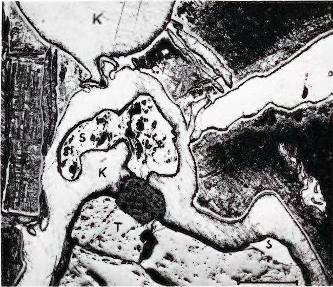
Figure 1683. Soroti (U.S.N.M. no. 1621). An angular chromite crystal (black) with associated monocrystalline troilite (T) and schreibersite (S). Shock-hatched kamacite (K) and acicular and martensitic plessite fields. Etched. Scale bar 400 \mu . (Henderson & Perry 1958: plate 19 – a different interpretation is given by them).
