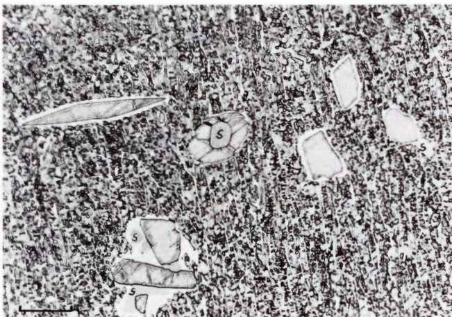
Figure 1687. South Byron (Chicago no. 2553). Fine kamacite spindles with schreibersite particles (S) in an almost unresolvable duplex \alpha + \gamma matrix. Etched. Oil immersion. Scale bar 10 \mu .
