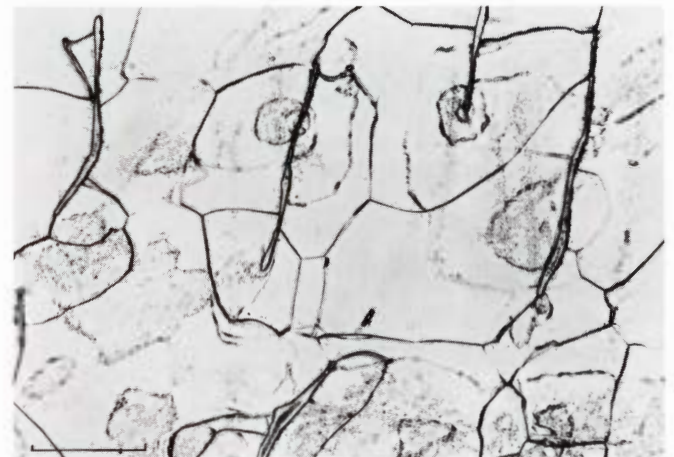
Figure 1672. Social Circle. (U.S.N.M. no. 1675). Grain growth with successive growth lines indicating several periods of rest. Distorted taenite lamellae vertically across the picture. Etched. Scale bar 100 \mu . See also Figure 220.
