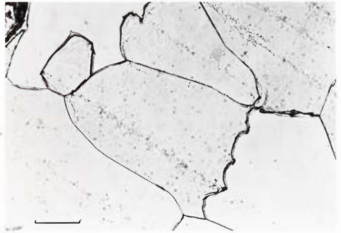
Figure 1671. Social Circle. Detail of Figure 1670. Indistinct remnants of parallel shear zones, probably Neumann bands. Grain growth restricted by fine \gamma -particles on the boundaries. Etched. Scale bar 40 \mu .
