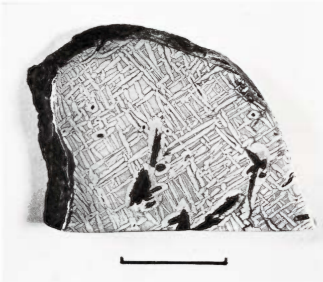
Figure 1704. Tambo Quemado (U.S.N.M. no. 1572). An artificially reheated medium octahedrite of group IIIB. The schreibersite skeleton crystals (black) are enveloped in swathing kamacite. Deep-etched. Scale bar 20 mm.
