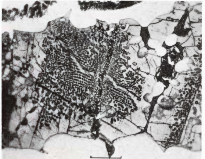
Figure 1708. Tambo Quemado (U.S.N.M. no. 1572). A phosphide which was associated with terrestrial oxidation products and upon artificial reheating formed complex melts. Etched. Scale bar 40 \mu . (Perry 1950: volume 9.)
