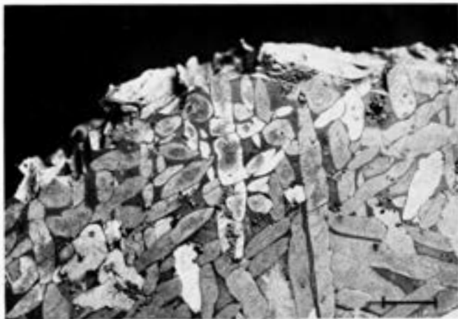
Figure 1713. Tanakami Mountains (Tokyo). A coarse octahedrite of group III E, a group related to III A-B. Note the swollen kamacite lamellae. The sample is weathered and shows small corrosion blisters that formed after finishing the polished section. Deep-etched. Scale bar 5 mm. (Courtesy Sadao Murayama.)
