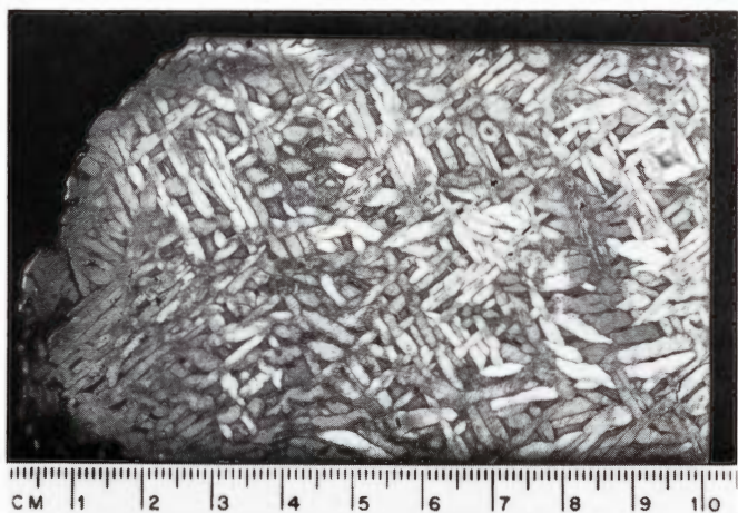
Figure 1700. Staunton (Tempe no. 155a of 659 g). A coarse octahedrite of group IIIE and related to Rhine Villa and Willow Creek. Note the swollen kamacite lamellae. Deep-etched. Scale in centimeters. (Courtesy C.B. Moore.)
