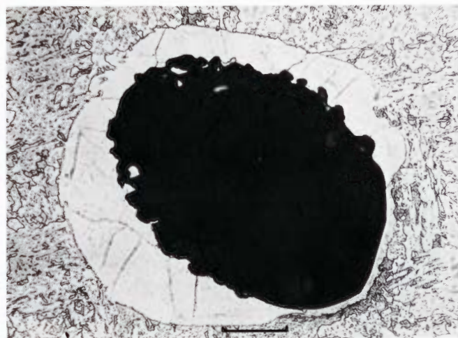
Figure 1809. Tucson (Ring mass) (U.S.N.M. no. 368). The larger silicates are globular or have ragged reentrant edges or combine both forms at once. The rim of swathing kamacite shows several subboundaries. The matrix is indistinctly duplex. Etched. Scale bar 40 \mu .
