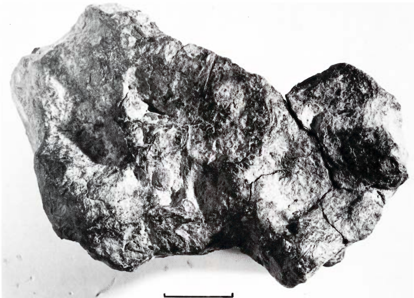
Figure 1819. Twin City. Main mass of 5.1 kg with deep, corroded fissures which upon sectioning turn out to follow primary austenite grain boundaries. Scale bar approximately 3 cm.
