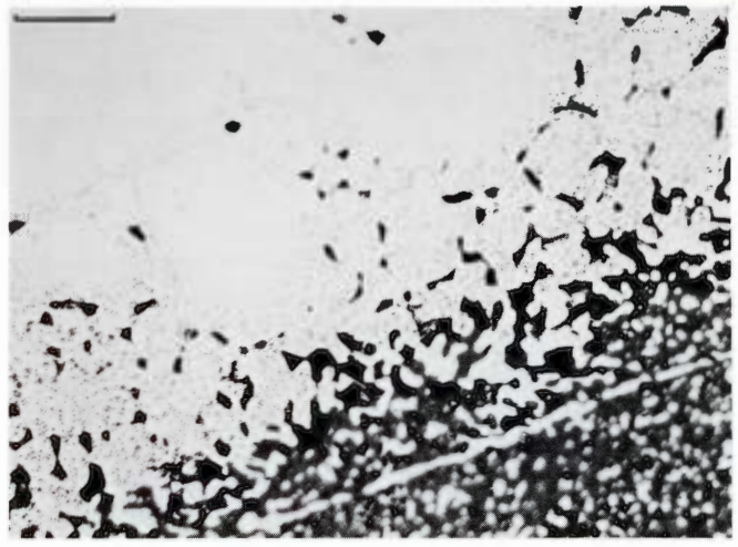
Figure 1816. Tucson (Carleton mass). Detail of Figure 1815 showing the edge of the inclusions. High temperature reaction products, comprising oxides, sulfides and glasses, occur at grain boundaries and, partially, within the metallic matrix. Polished. Oil immersion. Scale bar 20 \mu .
