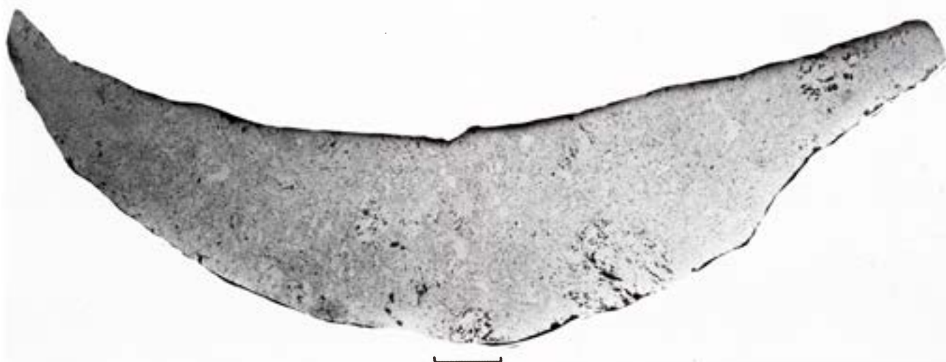
Figure 1801. Tucson. A crescent-shaped slice of 737 g from the Carleton mass (U.S.N.M. no. 757). The silicates (black dots) occur very irregularly over the section. Etched. Scale bar 20 mm. S.I. neg. 1334A.
