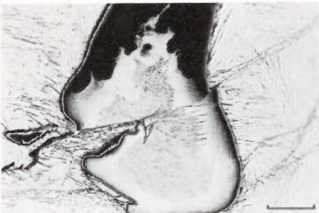
Figure 1848. Veliko-Nikolaevsky Priisk (Moscow no. 761). A plessite field which has been sheared and slightly displaced. A dense grid of slipplanes is visible in the taenite. Compare Figures 110 and 1849. Etched. Scale bar 30\ \mu .
