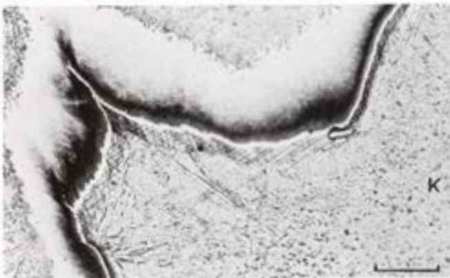
Figure 1849. Veliko-Nikolaevsky Priisk (Moscow no. 761). Detail of a taenite-kamacite (K) interface. The deformation grid in the taenite is particularly well observed on the tapering interface that has become exposed after the kamacite was partly etched away. Scale bar 30\ \mu .
