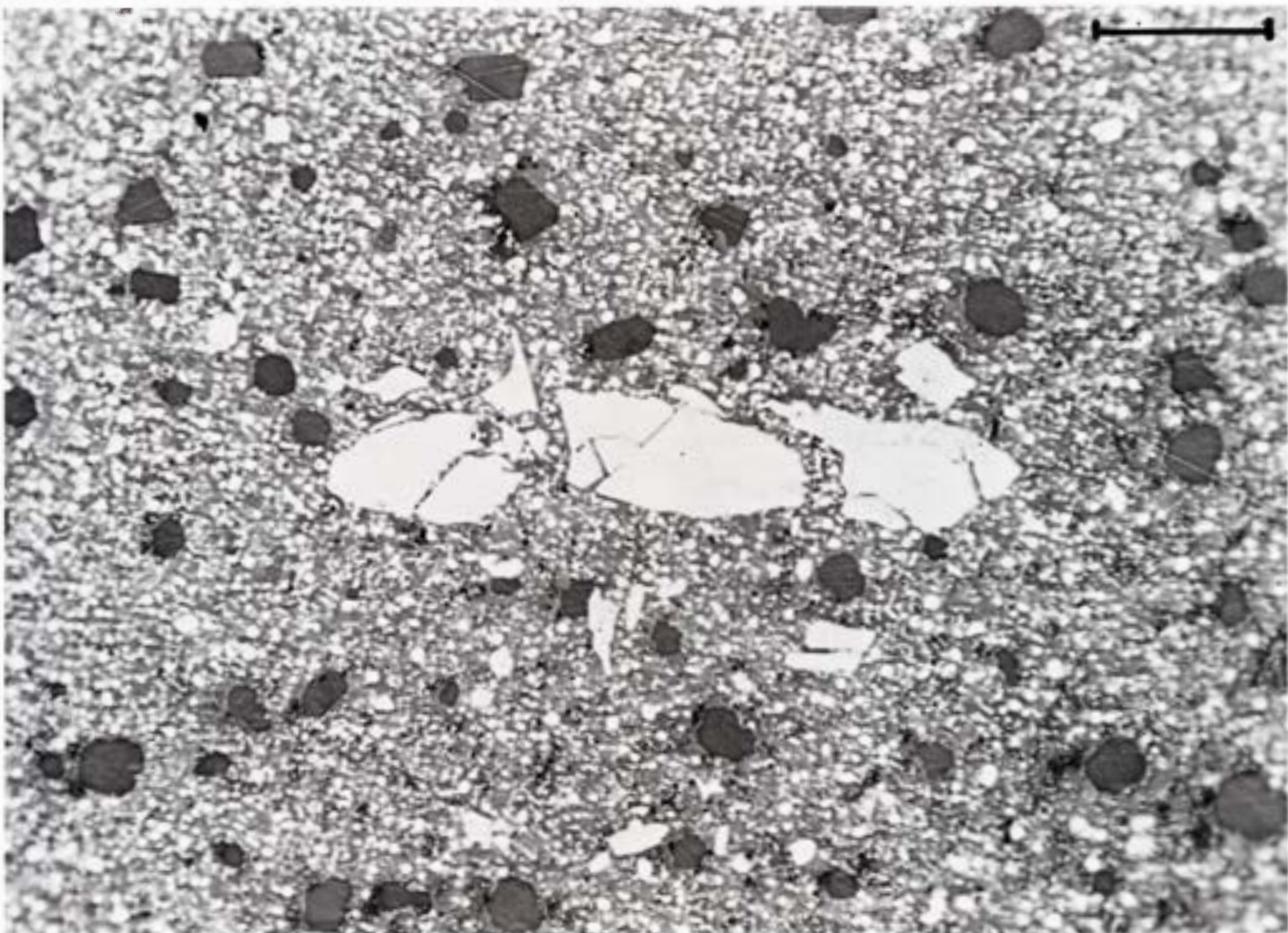
Figure 1841. Uwet (U.S.N.M. no. 601). Detail of shock-melted troilite nodule. Centrally a shattered schreibersite fragment torn loose from the troilite-kamacite interface. Daubreelite fragments (black) are dispersed in the sulfide (gray)-iron (white) eutectic. Polished. Scale bar 30 \mu .
