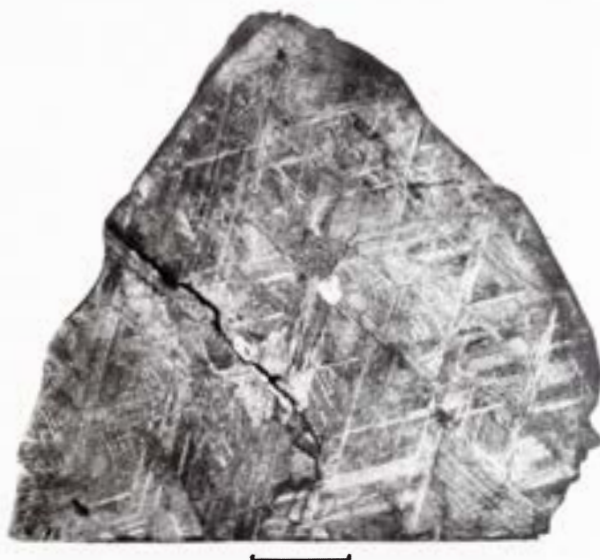
Figure 1827. Uegit (Rome). A medium octahedrite that probably belongs to group IIIA. Deep-etched. Scale bar approximately 2 cm. (From Millosevich 1924.)
