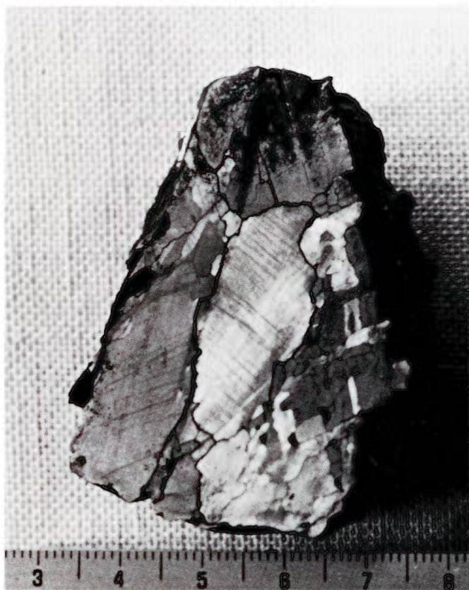
Figure 1828. Union County (Amherst). One of the largest preserved fragments, weighing 225 g. Coarse kamacite grains alternate with lamellar parts, and the whole structure is cold-worked and deformed. Deep-etched. Scale in centimeters.
