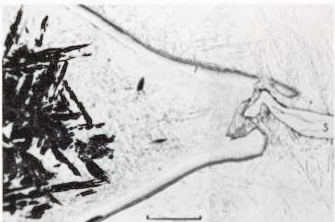
Figure 1846. Veliko-Nikolaevsky Priisk (Moscow no. 761). Shock-hatched kamacite and schreibersite in a grain boundary. Typical plessite field with martensite developed parallel to the bulk Widmanstätten pattern. Etched. Scale bar 50\ \mu .
