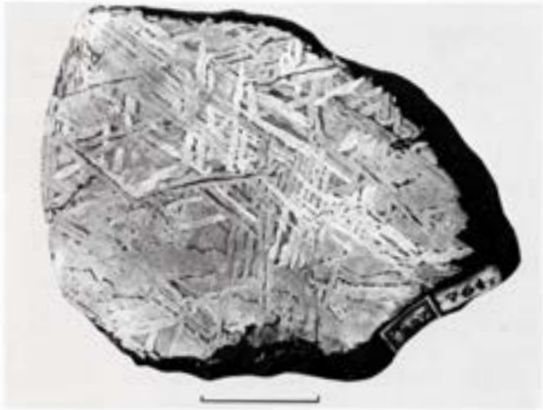
Figure 1845. Veliko-Nikolaevsky Priisk (Leningrad no. 237). A shocked medium octahedrite which probably belongs to group IIIA. Several distorted Reichenbach lamellae are seen (black streaks). Deep-etched. Scale bar 20 mm.
