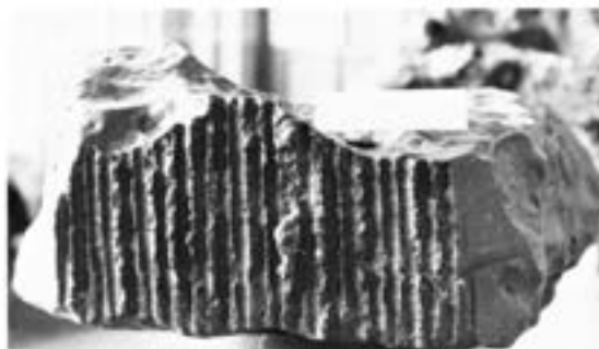
Figure 2026. Zacatecas (1792). The main mass as exhibited in Tacuba No. 5, Old School of Engineering, Mexico City. The parallel drill holes indicate how a – roughly – 200 kg endpiece was removed by Burkart in the 1830s. White ruler is 15 cm long.
