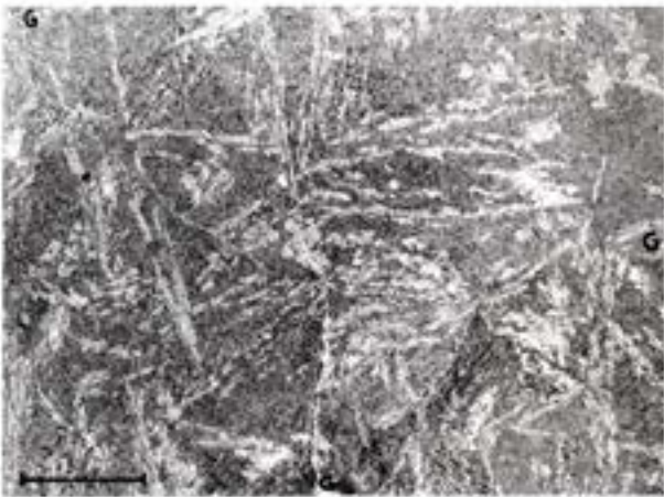
Figure 2022. Ysleta (New York no. 271). An anomalous meteorite of ataxite appearance. At high temperature it was composed of centimeter-sized taenite crystals. Three grains meet here near center. Grain boundaries G-G are narrow kamacite veins. Etched. Scale bar 2 mm.
