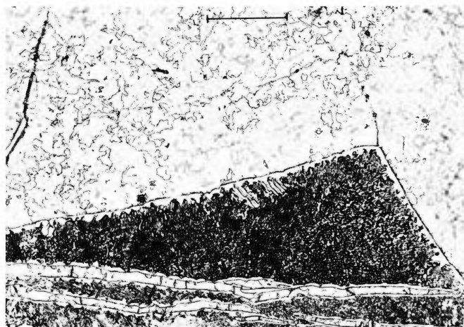
Figure 2018. Youndegin. The Mooranoppin fragment No. 1 (U.S.N.M. no. 1609). This sample has been artificially reheated. The kamacite is converted to unequilibrated \alpha_2 and the plessite fields are diffuse. Etched. Scale bar 100 \mu .
