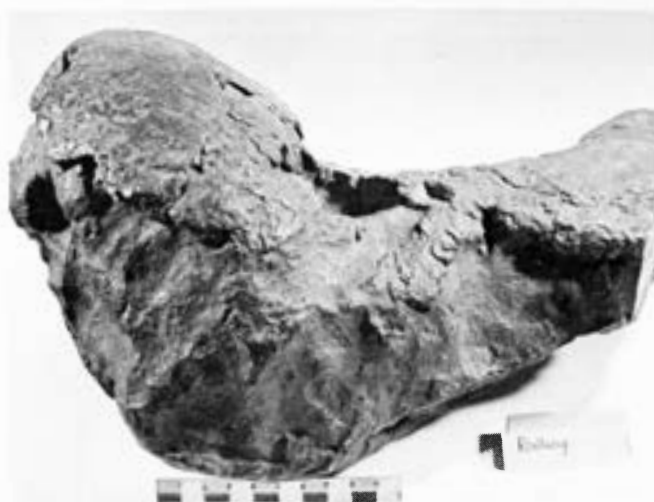
Figure 2077. Gibeon (Railway A) (Pretoria). A violently deformed fragment of the Gibeon shower. Twisted, necked and over-folded structures. Ruler in centimeters.
