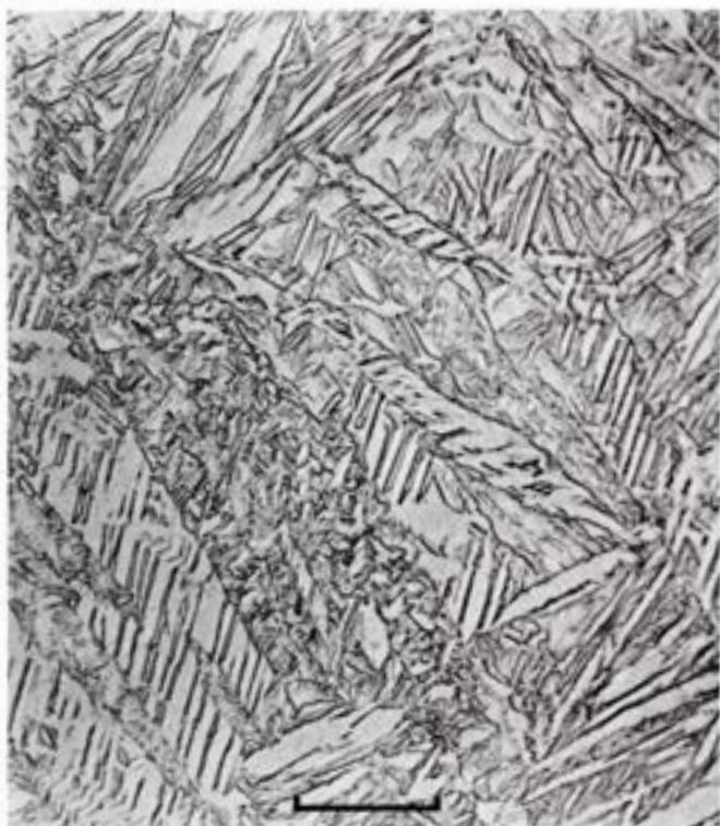
Figure 2079. Gibeon (Ganigobis). The hatched \epsilon -structure is shock-hardened to a Vickers hardness of 280 \pm 20 (100 g load). The high hardness is the combined effect of a high dislocation density and an extreme subdivision of the originally homogeneous kamacite crystal. Etched, Oil immersion. Scale bar 20 \mu .
