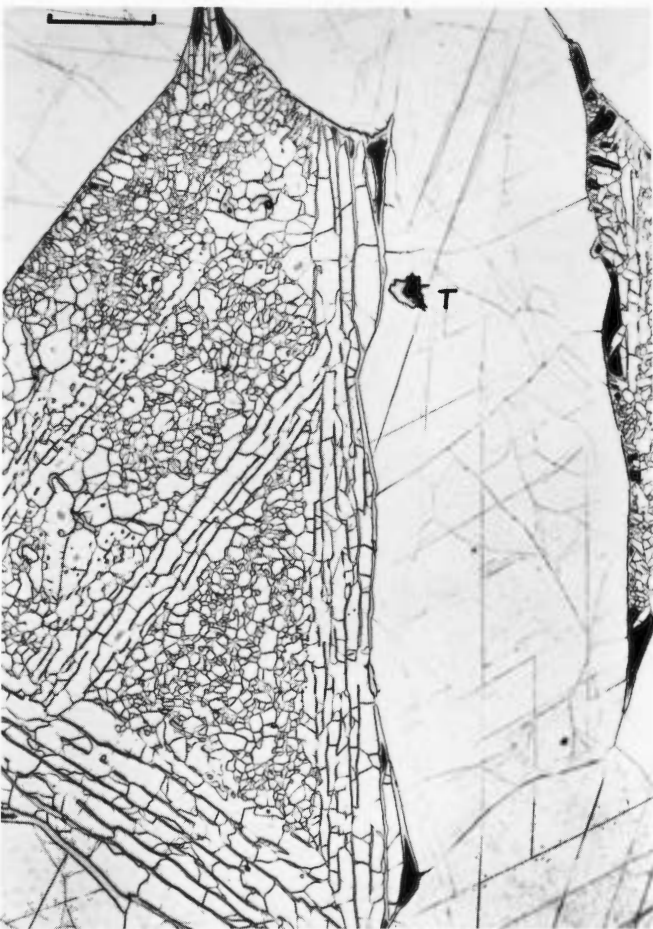
Figure 2054. Aswan (Cambridge No. 672). A large composite comb and net plesite field with numerous irregular schreibersite precipitates. The kamacite shows subboundaries and degenerate Neumann bands, compare Figure 2057. At T, a shock-melted schreibersite-troilite-daubreelite aggregate. Etched. Scale bar 0.5 mm.
