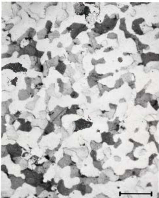
Figure 2075. Gibeon (Kamkas). Enlarged part of the eutectic in Figure 2074. White is unequilibrated kamacite, gray in shadings is polycrystalline troilite. Polished. Partly crossed Nicols. Scale bar 50 \mu .
