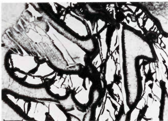
Figure 2050. Canyon Diablo (Albuquerque) (Institute of Meteoritics, Albuquerque). A coarse octahedrite of group I. Cohenite (white) has been thermally altered and is enveloped in black bainitic rims. Etched. Scale bar 0.5 mm.
