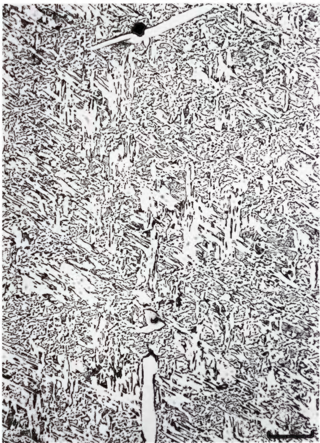
Figure 2063. De Hoek (Copenhagen). Occasional kamacite spindles occur in a Widmanstätten arrangement inside the grains. Sometimes they have been nucleated by phosphate crystals, as in this case above. The spindles shown are unusually wide for De Hoek, probably because they have been cut almost parallel to (111)_\gamma . Etched. Scale bar 100 \mu .
