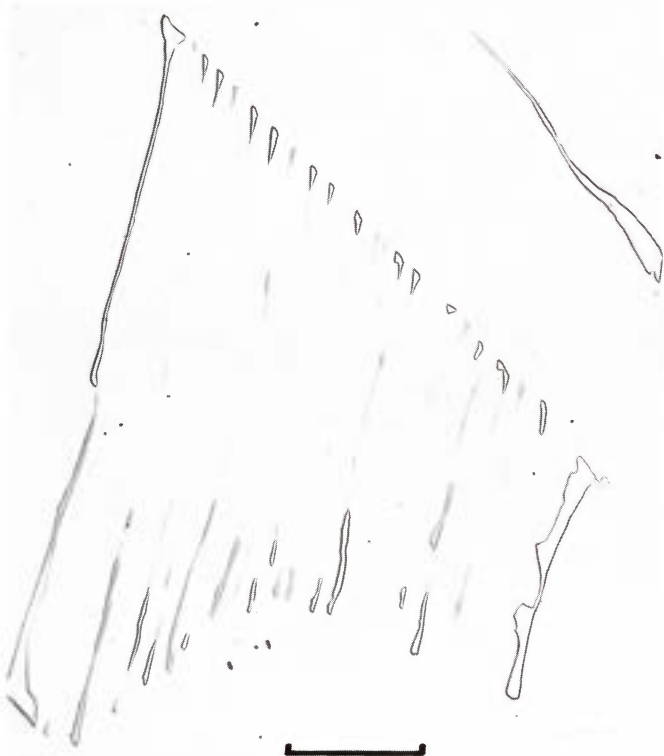
Figure 2065. Henbury (Gallipoli) (Tempe). A degenerate comb plessite field. This type is characteristic of medium octahedrites with less than about 7.5% nickel. Lightly etched. Scale bar 500 \mu .
