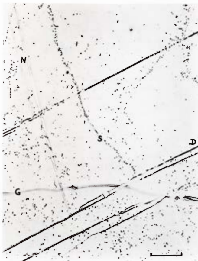
Figure 2057. Aswan. Tempered kamacite. A grain boundary (G) with phosphide precipitates is slightly out of focus. Decorated Neumann bands (D) run obliquely across, and late Neumann bands (N) are also seen. A subboundary (S) is mainly visible because of its micron-sized phosphide precipitates. Etched. Scale bar 50\ \mu .
